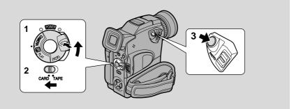
You can record still images onto a memory card. In addition to the still images you record directly onto the memory card, you can record images from a tape in the camcorder, or images input via the DV terminal or AV terminal onto the memory card.
